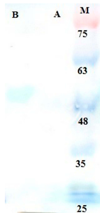
Figure 2 Western blot analysis of purified recombinant protein of \alpha -toxin-6 \times His tags. M: prestained Protein Ladder (Sinaclon, Iran). Lane A: Negative control E. coli strain BL21 (DE3). Lane B purified recombinant protein of E. coli BL21 (DE3) transformed with pET28a/ \alpha -toxin-6 \times His tags shows one band at 48 kDa.
