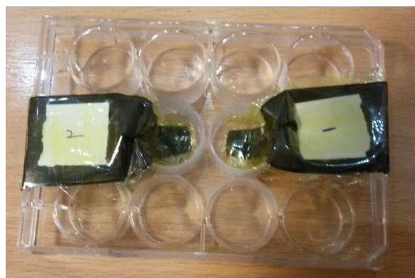
Figure 1: Dose verification using TLD-100 dosimeters.
