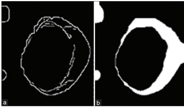
Figure 8: Effect of dilation operation. (a) Before and (b) after dilation
