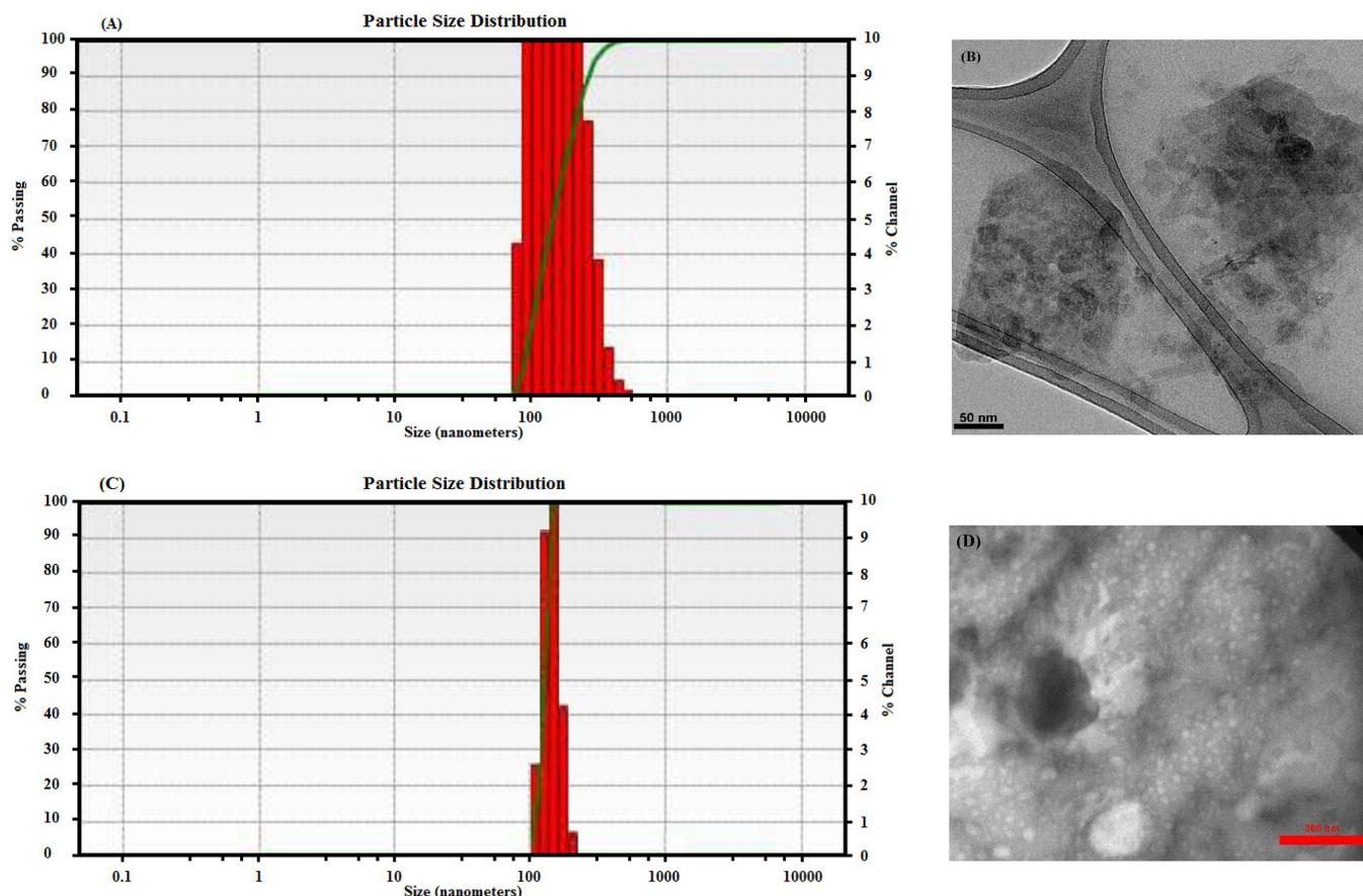
**Figure 3.** DLS and TEM results of PHEMA-st-PEGDA (A and B) and NH-MTX (C and D) at pH 7.4.
